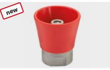
Hardened stainless steel. 3 x lateral front jets 15  $^\circ$  and centric front jet. Max. 500 bar /100  $^\circ C$
