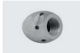
1/2" F. 6x 75° +1x 0°. 30-100 l/min. For \text{R} \text{ } \varnothing 100-200 mm. Outside \varnothing 40 mm. \text{g} 281 g.
