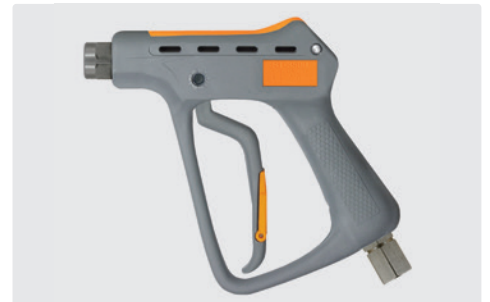
Professional high-flow gun. Stainless steel. Industrial high pressure cleaning and jetting gun for municipal cleaning and other industrial cleaning tasks. Valve piston hardened stainless steel. Swivel stainless steel. Max. 350 bar / 200 l/min / 150 °C
