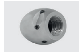
3/4" F. 6x 75° +1x 0°. 30-100 l/min. For \text{R} \text{ } \varnothing 120-250 mm. Outside \varnothing 50 mm. \text{g} 567 g.
