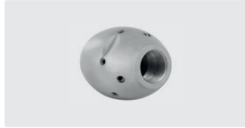
3/8" F. 6x 75° 3x 30° +1x 0°. 30-100 l/min. For \text{R} \text{ } \varnothing 100-200 mm. Outside \varnothing 35 mm. \text{g} 314 g.
