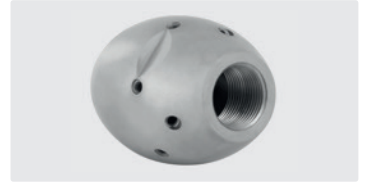
3/4" F. 6x 75° 3x 30° +1x 0°. 100-250 l/min. For \text{R} \text{ } \varnothing 150-300 mm. Outside \varnothing 50 mm. \text{g} 1,367 g.
