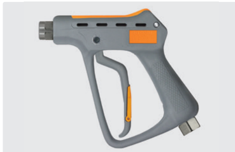
Professional high-flow gun. Stainless steel. Industrial high pressure cleaning and jetting gun for municipal cleaning and other industrial cleaning tasks. Valve piston hardened stainless steel. Max. 350 bar / 200 l/min / 150 °C
