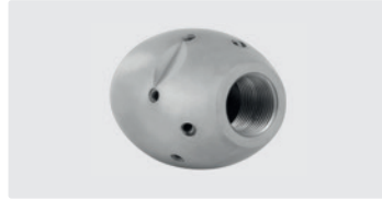
1/2" F. 6x 75° 3x 30° +1x 0°. 80-140 l/min. For \text{R} \text{ } \varnothing 120-250 mm. Outside \varnothing 40 mm. \text{g} 630 g.
