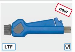
Professional gun with locking in opened position and coupling ST-3100. Stainless steel. Field of application: foam and rinsing applications in the food industry etc. Industry standard. Max. 24.5 bar / 120 l/min / 100 °C
