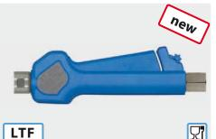
Professional gun with progressive closing system and locking in opened position. Stainless steel. Field of application: foam and rinsing applications in the food industry etc. Industry standard. Max. 24.5 bar / 120 l/min / 100 °C
