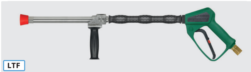
1/2" F. Stainless steel. Longcast lance 350 mm with insulation ST-29 Cool & Compact 330 mm, gun easyfarm365+, grip aside and nozzle protector made out of plastic without nozzle. Max. 250 bar / 60 l/min / 100 °C
