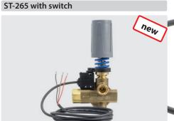
⊕ = Inlet 3/8" F. ⊕ = Outlet 3/8" F. BP = Bypass 3/8" F. Ball check valve. Unloader valve with pressure switch (IP65) and cable 1,200 mm. Max. 350 bar / 80 °C
