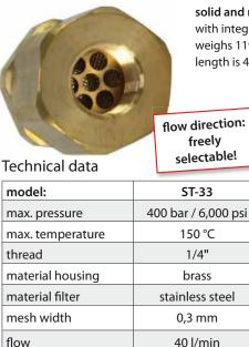
solid and robust: the brass housing with integrated stainless steel filter weighs 119 grams and the total length is 45.6 mm
