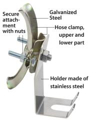
Simple mounting on the hose: By loosening the two screw connections (Hex 10) on the clamp, the hose can be easily clamped.
