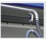
Easy handling with the spring balancer: Cables or hoses are kept off the ground and protected. No trip hazards when loading the vehicle.
