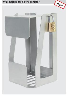
Stainless steel. Two-part with cover. 4 mounting holes for wall mounting,  $\emptyset$  8.5 mm. Delivery without lock. H/W/D = 320/198/180 mm. 2 kg
