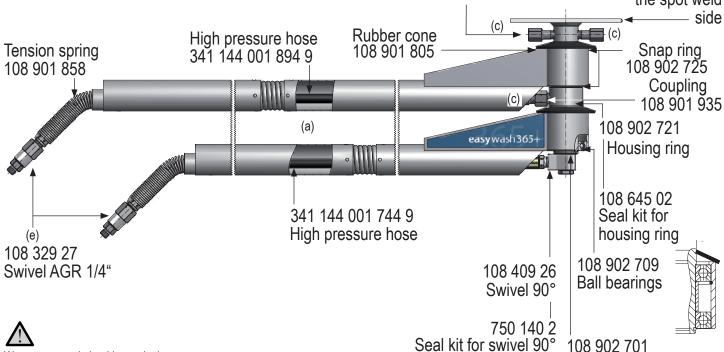
We recommend checking swivelconnections once a year for normal wear and tear.
