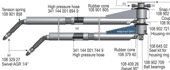
We recommend checking swivelconnections once a year for normal wear and tear.
